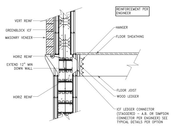
8" TO 6" WALL W/BRICK LEDGE; FLOOR PERPENDICULAR TO WALL
